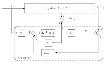
To find  $L_{obs}$ , we focus on system with "input" u(t) and "output"  $\varepsilon_x(t) = \hat{x}(t) - x(t)$ .
