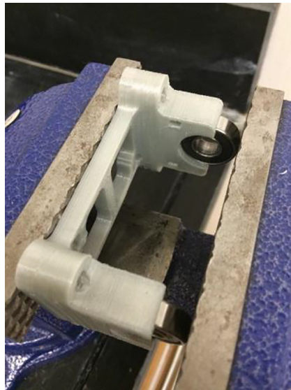
Fig. 2. The use of a vice or vice grips to press fit bearings into 3-D printed plastic parts.
