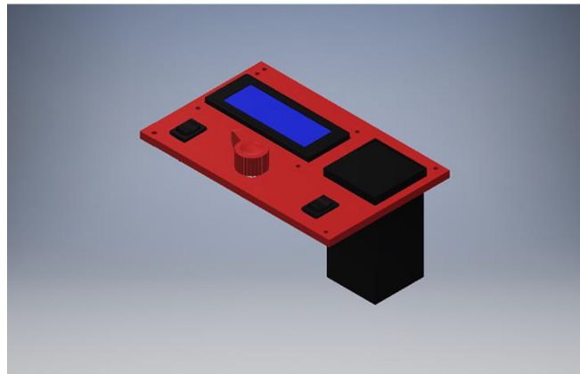
Fig. 39. Mounting LCD, Heater Control, Switches and Rotary Encoder with knob to front cover.
