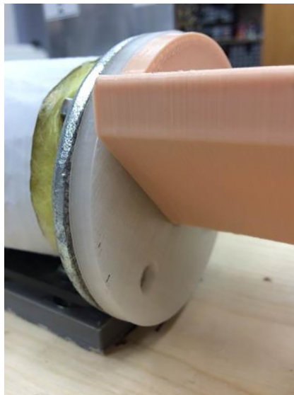
Fig. 18. Insulation for hopper.
