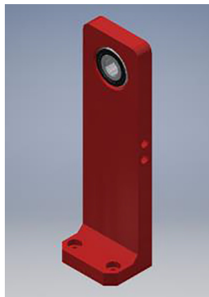
Fig. 89. Bearing in opposite bearing tower.
