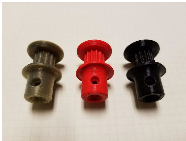
Fig. 111. Comparison between printed products from recycled PLA (Made, left), virgin PLA (Made, middle) and virgin PLA (Purchased, right).
